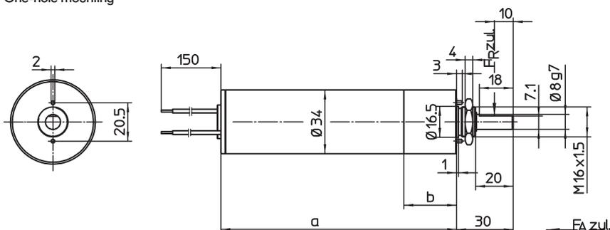
Mounting nut for one-hole mounting must be tightened up to 10 Nm.
